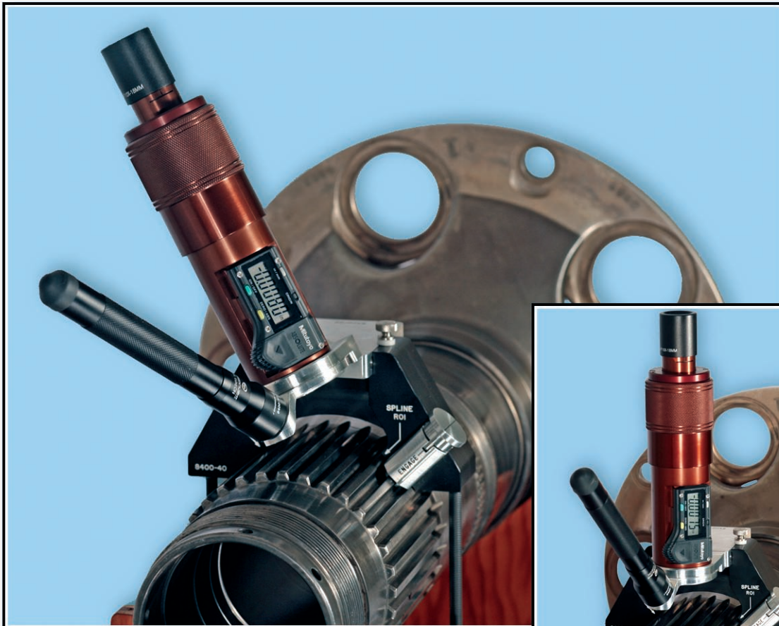
Micrometer is upright for shaft inspection (inset), or tilted perpendicular to region of interest ("SPLINE ROI") on spline faces.
